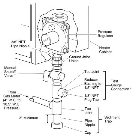
\* An A.G.A. design-certified manual shutoff valve with 1/8" NPT tap is an acceptable alternative to test gauge connection. Purchase the optional A.G.A. design-certified manual shutoff valve from your dealer. See *Accessory*, page 15.
